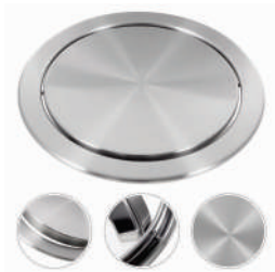
DWBN0043 & 44 Table Mount Dustbin-Lid 304 Stainless Steel DWBN0043 Diameter : 238mm Installation Required Size : 193(min)-223(max) mm DWBN0044 Diameter : 268mm Installation Required Size : 218(min) -248(max) mm
